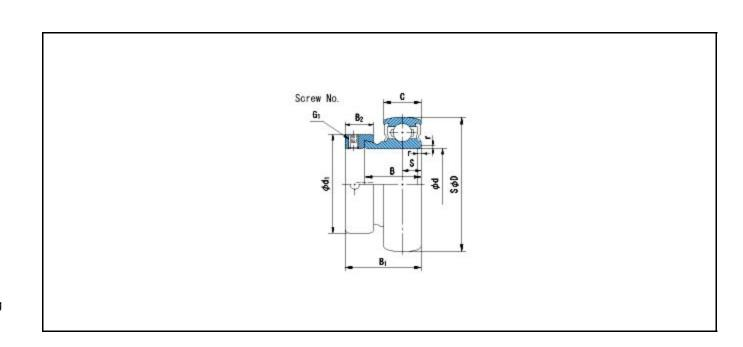
Basic Dynamic Load Rating Cr : 12800 N INNER RING OUTER RING
